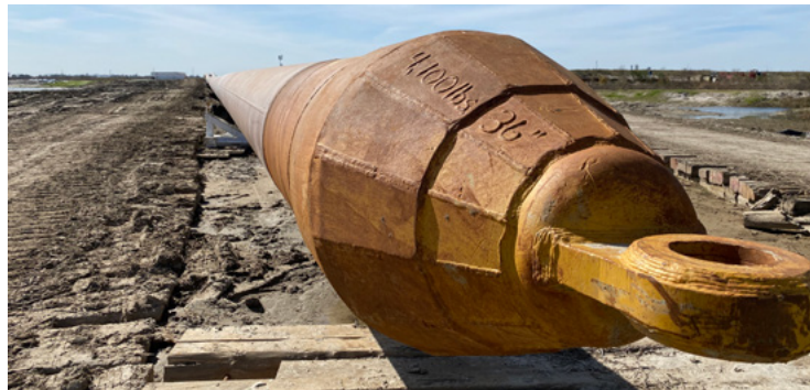
The two-ton reamer that cleared the pipeline path dozens of feet below the Ship Channel.
